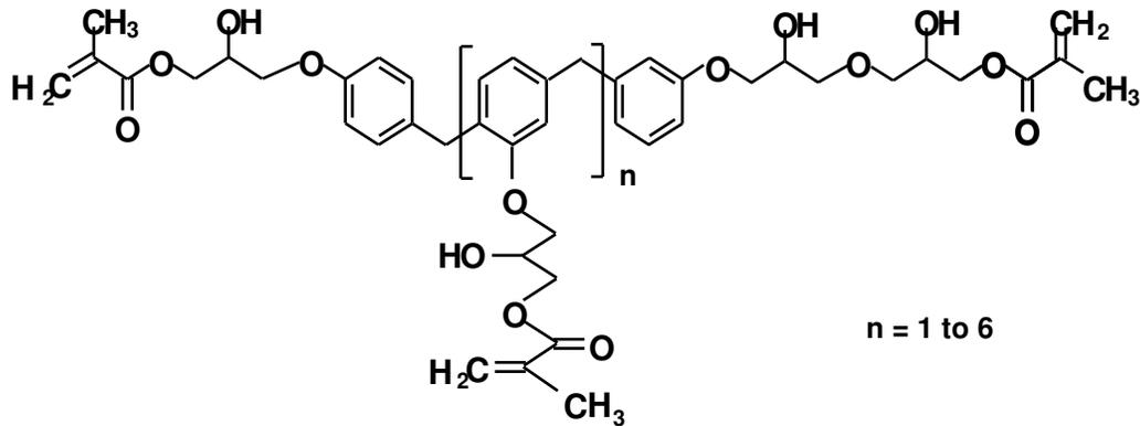
Figure 5. Epoxy Novolac Vinyl Ester Resin Structure
