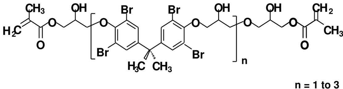
Figure 6. Brominated Epoxy Vinyl Ester Resin Structure
