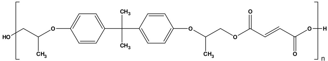
Figure 2. Bisphenol A Fumarate Polyester Resin Polymer Structure
