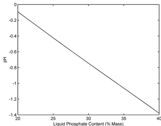
Figure 22. pH versus phosphate levels at 80 °C and 1.5 % sulfates
