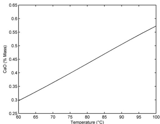
Figure 19. CaO vs temperature at 1.5 % sulfates & 30 % phosphates
