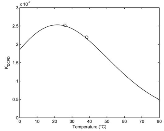
Figure 7. DCPD equilibrium constant versus temperature
