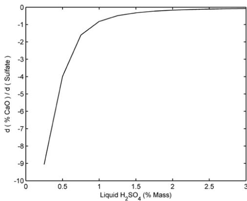
Figure 15. CaO ROC versus sulfates at 80 °C and 30 % phosphates
