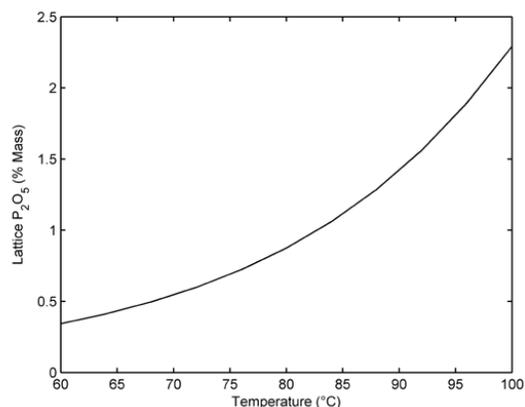
Figure 20. LL vs temperature at 1.5 % sulfates and 30 % phosphates
