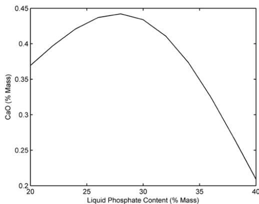
Figure 23. CaO versus phosphate levels at 80 °C and 1.5 % sulfates
