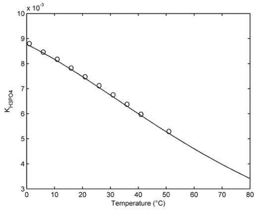
Figure 3.  $H_3PO_4$  equilibrium constant versus temperature
