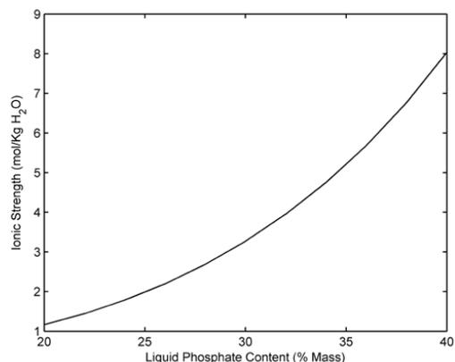
Figure 21. IS versus phosphate levels at 80 °C and 1.5 % sulfates
