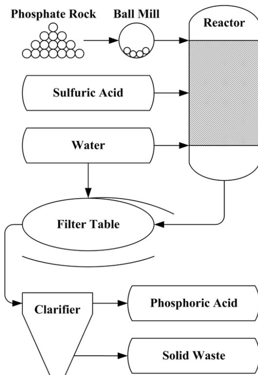
Figure 1. Phosphoric acid production by the dihydrate process
