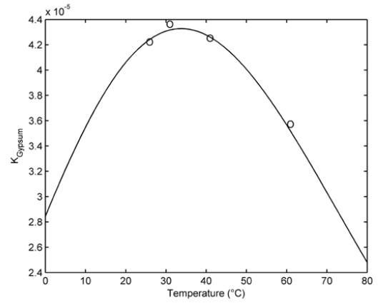
Figure 6. Gypsum equilibrium constant versus temperature
