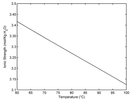
Figure 17. IS vs temperature at 1.5 % sulfates and 30 % phosphates
