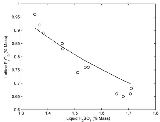
Figure 8. Lattice loss versus sulfates at 79  $^{\circ}C$  and 31 % phosphates
