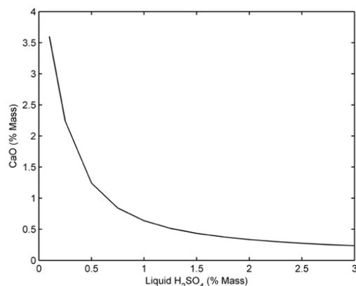
Figure 11. CaO versus sulfates at 80 °C and 30 % phosphates
