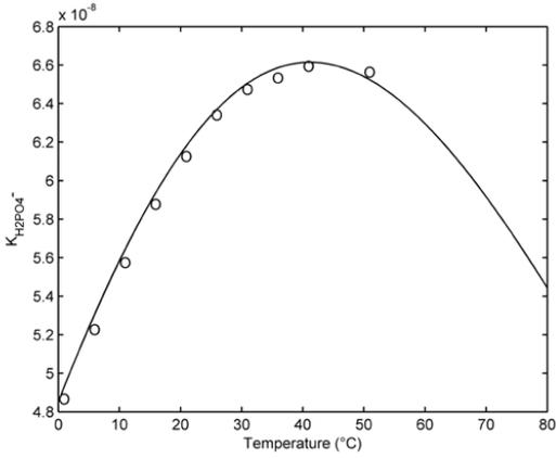
Figure 4.  $H_2PO_4^-$  equilibrium constant versus temperature
