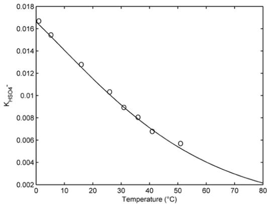
Figure 5.  $HSO_4^-$  equilibrium constant versus temperature
