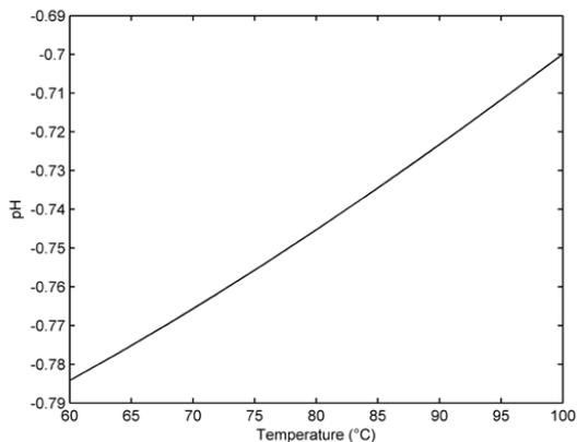
Figure 18. pH vs temperature at 1.5 % sulfates and 30 % phosphates
