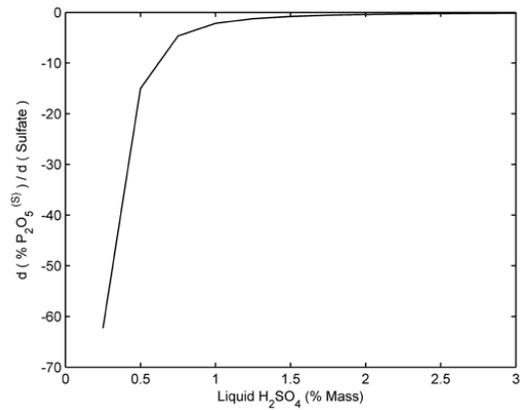
Figure 16. LL ROC versus sulfates at 80 °C and 30 % phosphates
