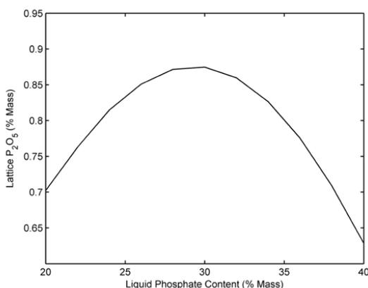
Figure 24. LL versus phosphate levels at 80 °C and 1.5 % sulfates
