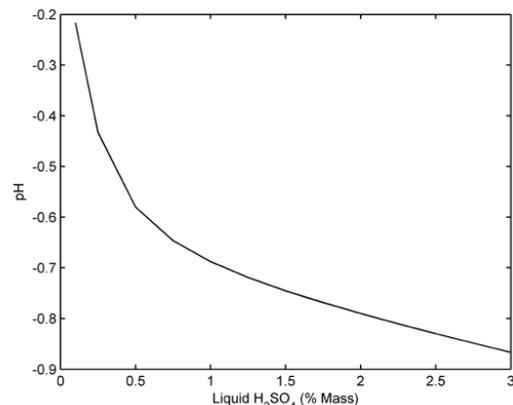
Figure 10. pH versus sulfates at 80 °C and 30 % phosphates
