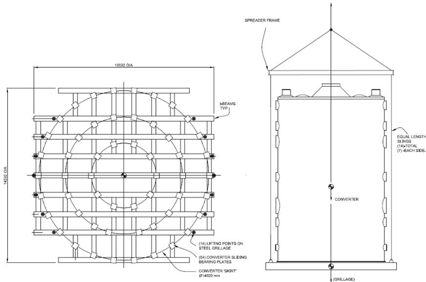
In practise, however, this turned out to be an impractical solution, so Bateman Engineering designed a new lifting arrangement for each converter, which could now be fully utilised in Durban South Africa, at the Madagascan port of Tamatave and on site.
