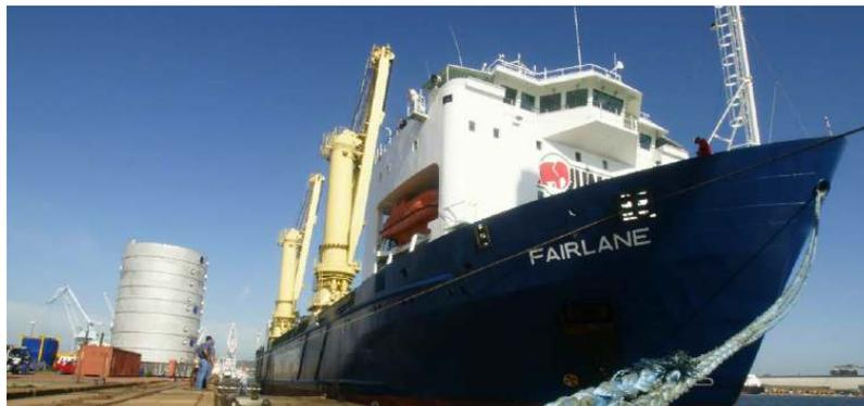
The preparations specifically required included the complete redesign and supply of the lifting arrangement of the converter, an area adjacent to the wharf had to be dredged to achieve 7.5m depth and the completed converters had to be moved closer to the edge AND had to be rotated by 90° for the ships cranes to reach the lifting arrangement. Much of this study work and preparation theory was concluded in conjunction with Jumbo Shipping’s professional team of engineers.
