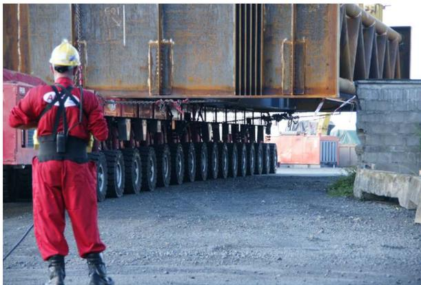
**Figure 12 : Moving the converter across the newly constructed bridge**
