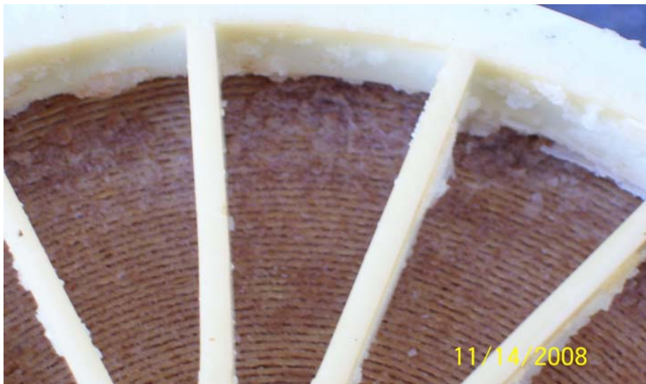
Figure 9 – RO Membrane fouled with various gyp-stack water precipitated salts.
