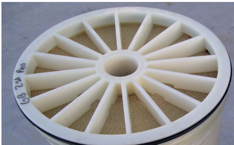
Figure 10: RO Membrane cleaned for re-use.
