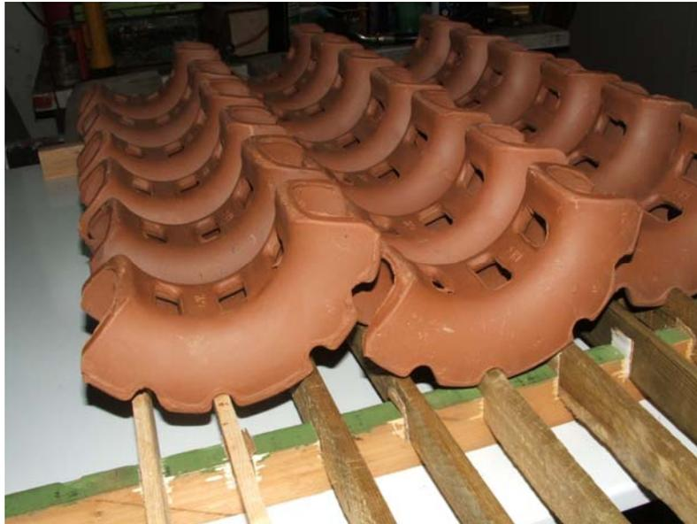
Ceramic support grids on ceramic beams and ceramic dome designs are accommodated by the packing system design with similar minimal losses across the interface.
