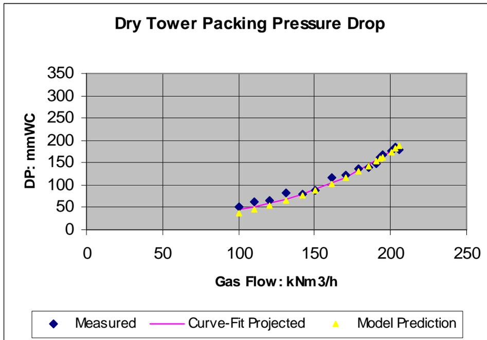
Using the same model, the quantity of packing required for the Bartow tower was predicted as 25 pieces per cubic foot of tower volume. Actual quantity used was 24.8 pieces per cubic foot. The pressure drop reduction was predicted as a 60% reduction from the standard saddles and actual has been > 80% reduction using the HP+ packing.
