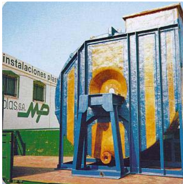
Figure 7. Phosphate Fertilizer Process Fan for 80°C (182°) P 2 O 5 Fumes
