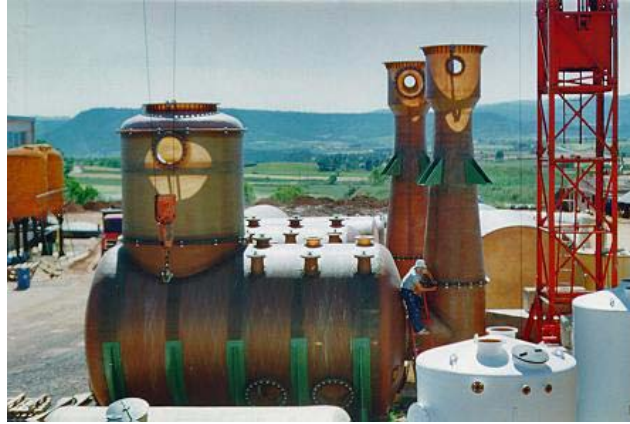
Figure 10. Venturi Scrubber for Ammonia and Hydrogen Sulfide
