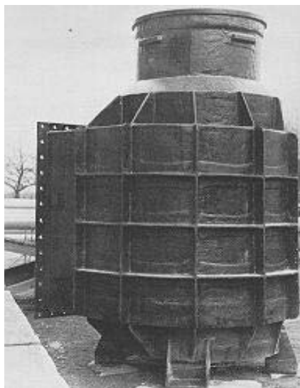
Figure 9. FRP Separator Recovers Phosphoric Acid from Waste Fumes
