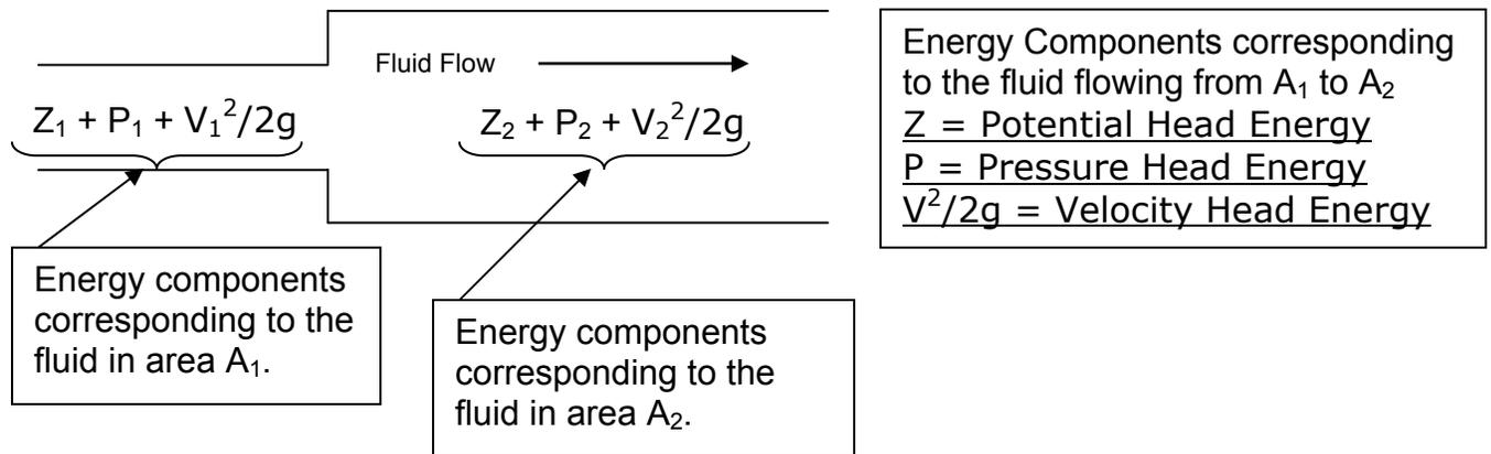
**Figure #2** – Bernoulli's Principle states that the sum of all forms of energy in a fluid flowing along a streamline is the same at any two points in that path. Therefore  $Z_1 + P_1 + V_1^2/2g = Z_2 + P_2 + V_2^2/2g$ .
