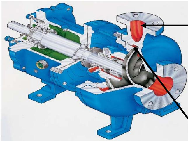
As the fluid exits the pump, the cross sectional area increases, the fluid velocity decreases thus decreasing the Velocity Head energy ( $V^2/2g$ ). With the reduced ( $V^2/2g$ ) the law of conservation of energy states that the Pressure Head energy must increase.
