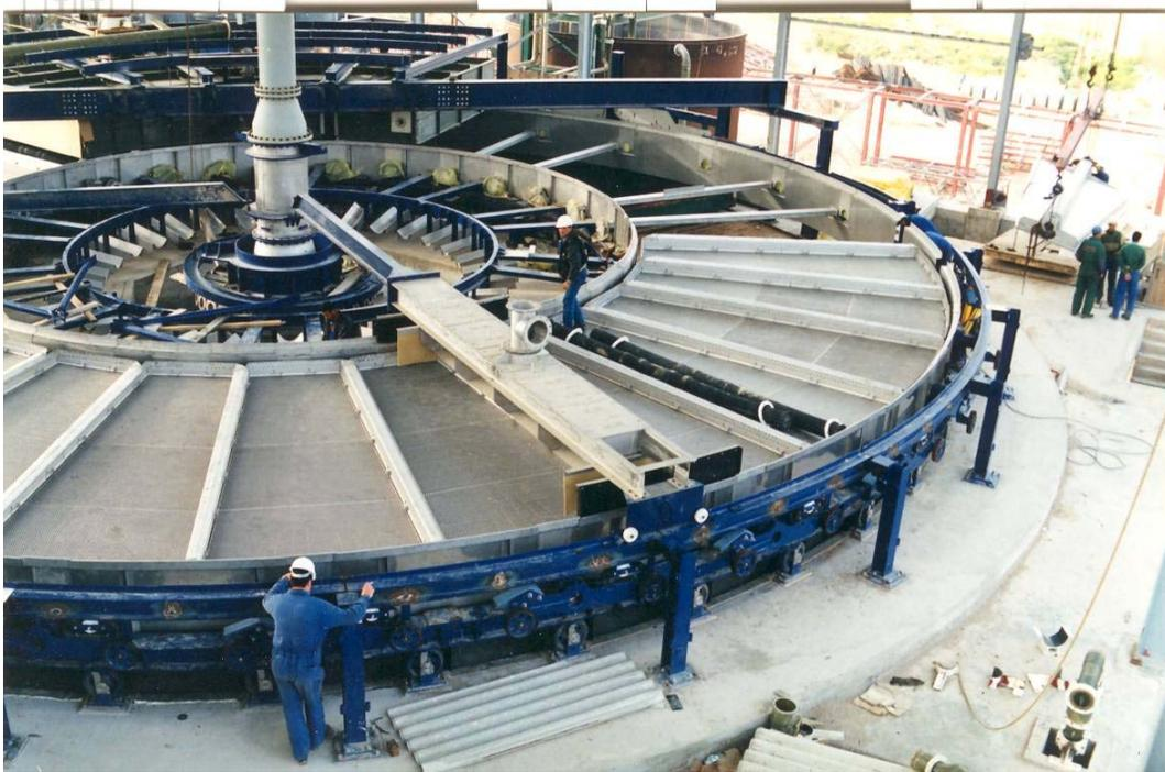
30-165EE Prayon filter (225 SQM in semi wet discharge) boosted up to 247 SQM (2660 SQF) in wet discharge for the OCP – BUNGE project.
