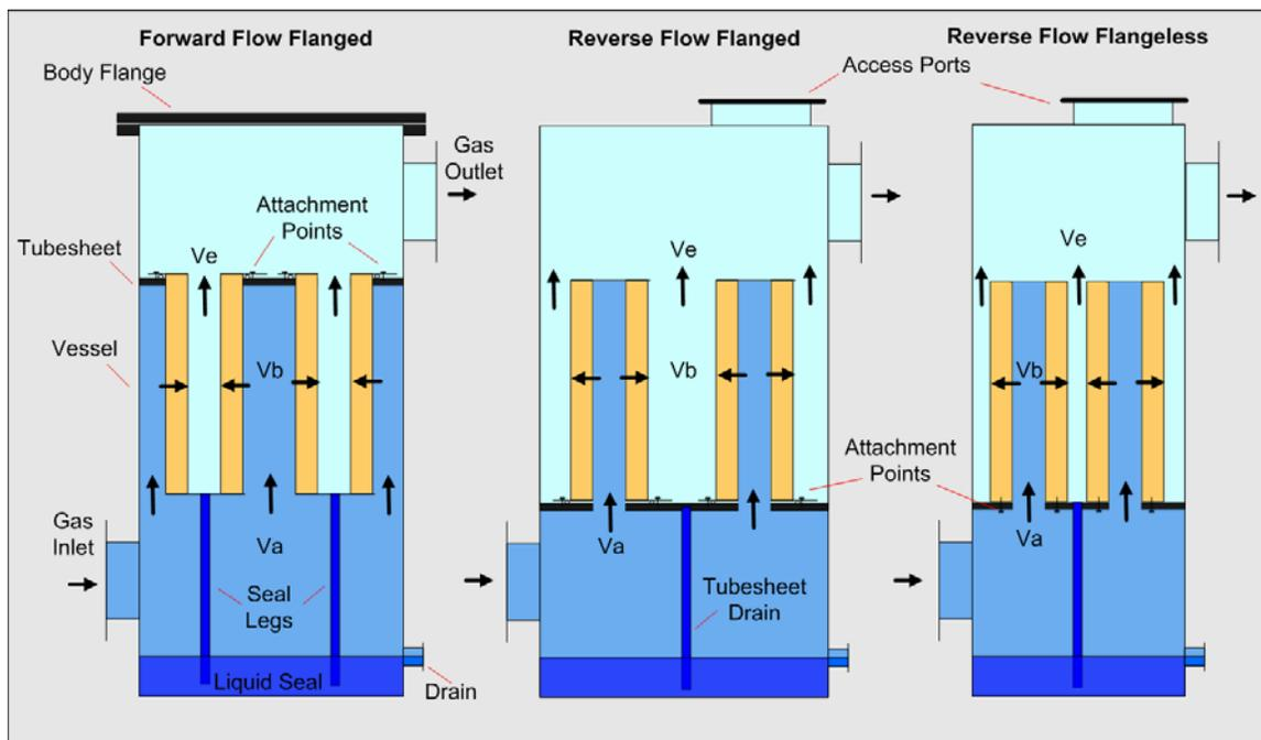
When choosing an installation style for a particular application, there are mechanical and maintenance tradeoffs. For example, because of higher gas throughput, cylindrical impaction fiber beds almost always use reverse-flow flanged style since this results in an optimum balance of gas velocities. Factors that influence installation style include large installations, corrosive processes and maintenance issues.
