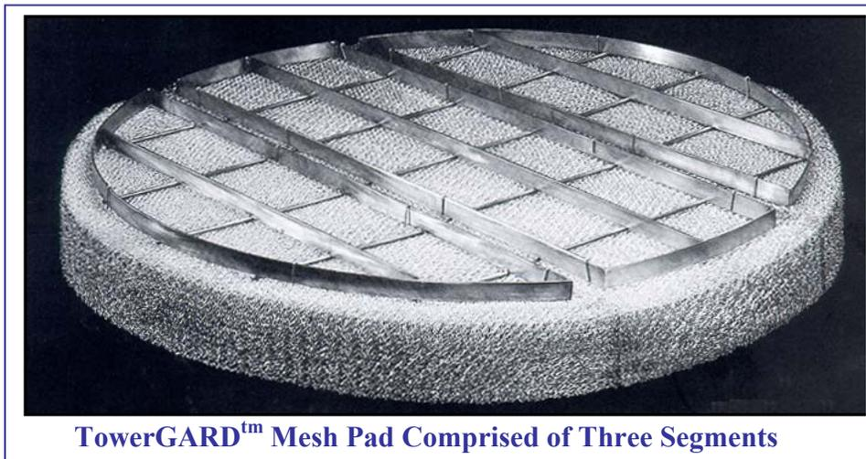
Since mesh pads are relatively low pressure drop devices (25 to 100 mm wc), it is important to ensure proper installation to achieve uniform velocity across the pad surface. Proper design of inlet and outlet duct locations are an often overlooked design principle. Sufficient clearances must be provided for introducing and removing gas from the pad otherwise poor flow distribution through the pad can lead to poor pad performance.
