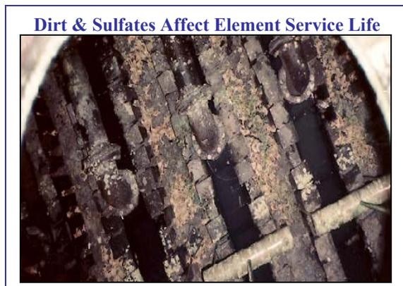
CK elements use a metal mesh structure with small diameter acid resistant glass fibers knitted together with the metal wires to increase the collection targets and thus small particle collection efficiency. The co-knit metal mesh collecting layer is considerably thicker and has a higher void fraction than the glass collecting layer used in standard CS elements. In severe plugging situations, CK elements operate much longer between cleanings than regular CS elements.
