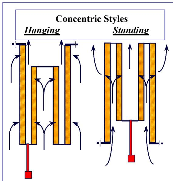
There are distinct advantages to this approach because use of concentric beds increases filtration area while using the same conventional bolting making retrofitting possible. The use of concentric elements can lead to lower pressure drop by as much as 30 to 50 percent depending upon element style and application. Increasing fiberbed area obtained when installing concentric beds often allows for increased gas flow and/or plant capacity at the same pressure drop across those elements.
