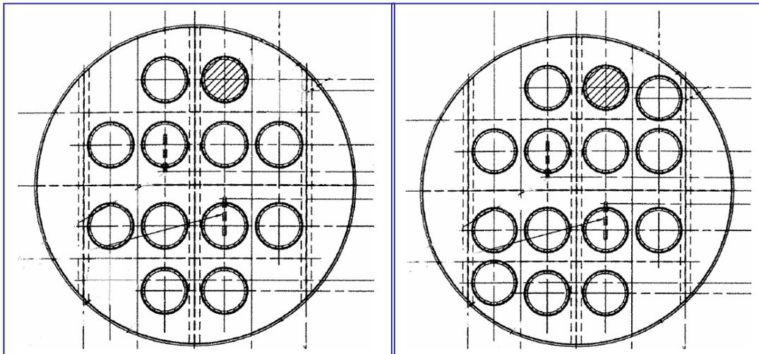
Two extra elements were installed on the existing tubesheet resulting in an 18 percent increase in overall bed area. The original blank (shown cross lined) was not used in case further capacity was needed. In the final tower, additional small diameter CS elements were installed to provide the proper design velocity to accommodate the plant rate increase.
