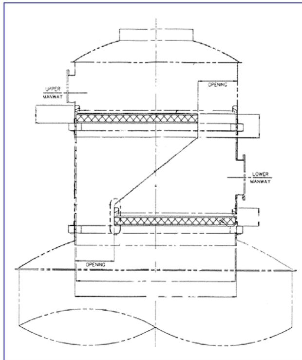
To assure proper operation, the openings around the Z-pad sections are designed to balance the gas flow through the two Z-pad sections.
