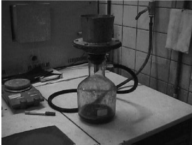
Figure 5 - Filtration test cell
