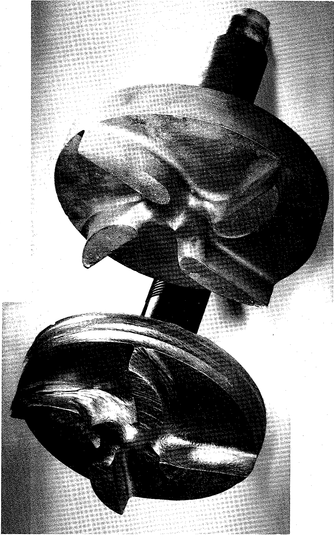
Low Velocity Test Comparisons Impervious Graphite vs SiC Impeller 120 Hrs. 3-5% Foundry Sand Impervious Graphite SiC Impeller 1200 Hrs. Impeller Fig. 4
